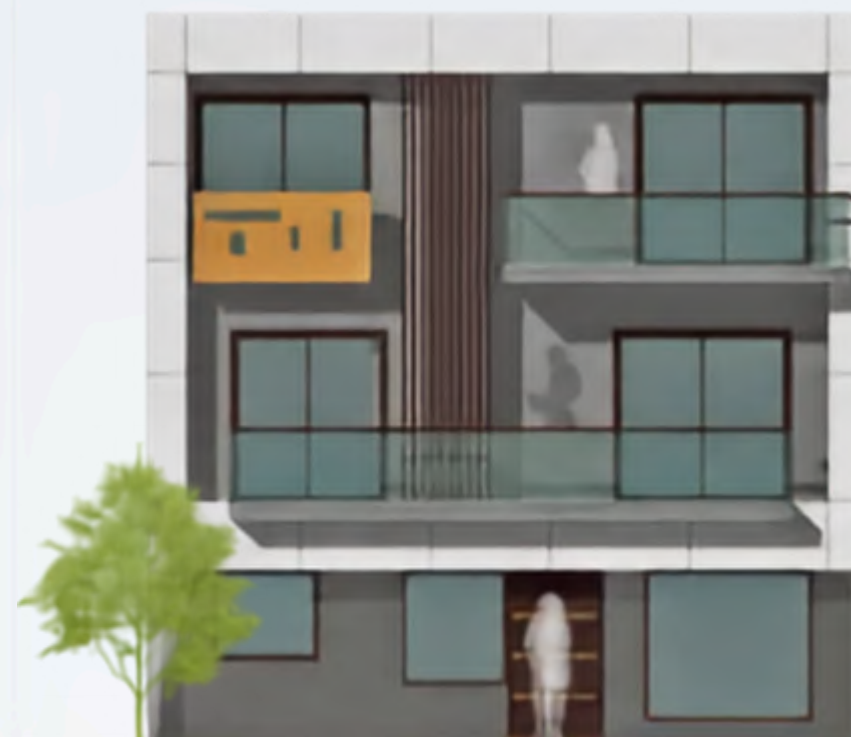
Toughened glass railing with timber handrail
